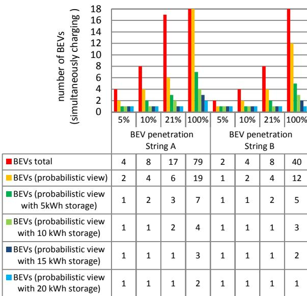
Figure 6. Maximum number of simultaneously charging BEVs from the grid – in worst case, with probabilistic view itself (arrival time at 18.00h, distribution of daily driven distances and confidence level 99.7%) or if the related charging stations are supported by battery storages
