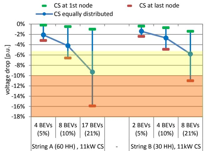
Figure 5. Range of the additional voltage drop on two strings caused by simultaneously charging BEVs using 11kW charging stations (CS) with different assumptions of the distribution of the connection points of the CS within the strings
