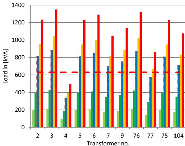
Figure 3. Maximum load on the transformer caused by peak loads of households (HH) by itself and including the load of charging BEVs (21%) with all BEVS charging simultaneously (Case A) and different power rating of the charging stations (same legend as Fig. 4).
