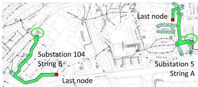
Figure 1. The additional voltage drop caused by BEVs is analyzed on two overhead power lines of the low voltage grid of a town in southern Germany – string A has a branched structure while string B is essentially a single line.
