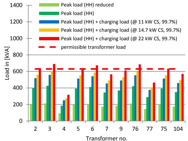
Figure 4. Maximum load on the transformer caused by peak loads of households (HH) by itself and including the load of charging BEVs (21%) with different power ratings of the charging stations using a probabilistic view (Case B – confidence level of 99.7%)
