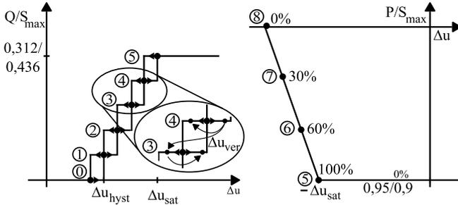
Figure 7: Improvement of the control characteristics by implementing hysteresis for reactive power control and predictive calculations for active power control
