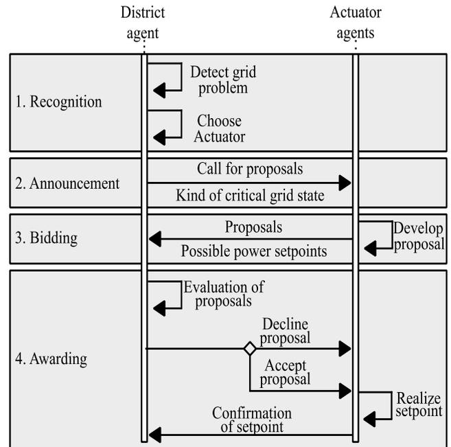
Figure 4: Phases of Contract Net Protocol to solve critical grid situations [10]
