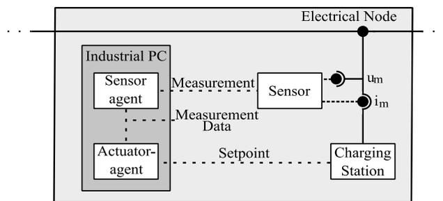
Figure 2: Configuration of an autonomous controller
