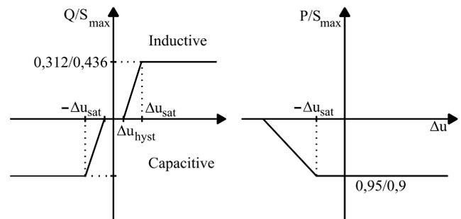
Figure 3: Autonomous, voltage dependent control of charging stations
