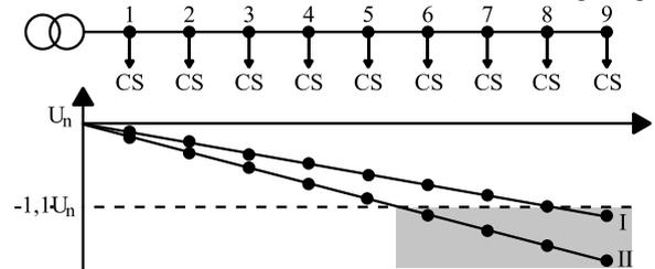
Figure 6: Scenarios for the analysis of coupling effects of several decentralized controllers
