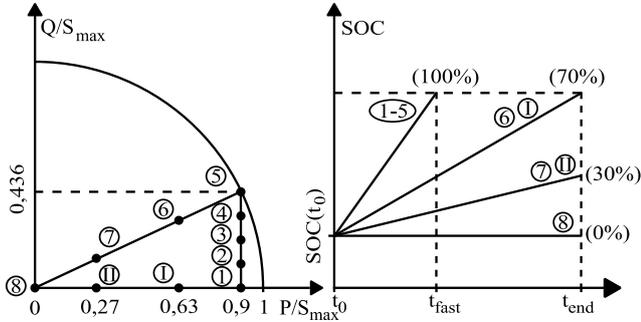
Figure 5: Left: Operating points of a charging station, Right: SOC of an electric car at different operating points of the charging station
