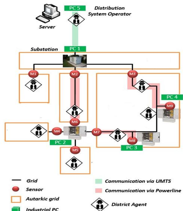
Figure 1: Hardware structure of a multi-agent system [4, p.2]
