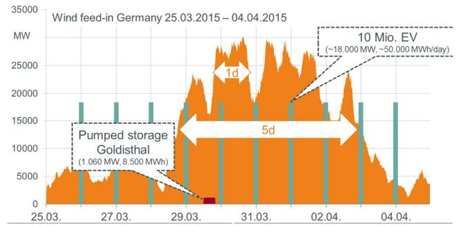
Figure 9. EV as power storage devices in comparison to a 2015 windfront infeed in Germany
