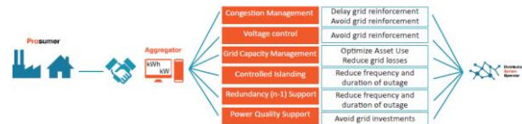
Fig 3: Aggregation services for the DSO
