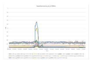
Figure 1 Supra harmonics in phase L2 at Substation A, significant levels of frequency 44 and 46 kHz originated from EV charging, work day 1
