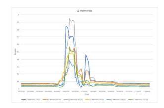
*Figure 4 Current harmonics in phase L2 at Substation A, order 3, 5, 7, 9, 11 and 13, work day 2*
