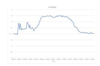
Figure 7 Voltage THD in phase L2 at Substation A, work day 1
