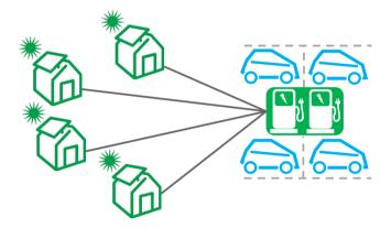
Figure 1. Charging current sharing in areal grids: Charging of electric vehicles with green electricity self-produced by the community
