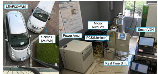
Figure 1. Experimental setup of the HIL.
