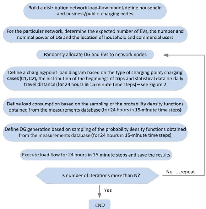
Fig. 3. Flowchart of the sequential Monte-Carlo algorithm basic steps.
