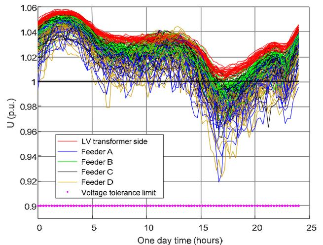
Fig. 8. Voltage profile in rural LV network in 2030, for the case of three-phase charging (7 kW charging power), fast EV growth and simulation case C1.
