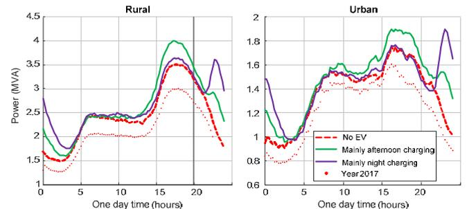
Fig. 6. Power-flow of urban and rural feeders in 2030 for fast EV growth and different simulation cases (3.6 kW charging power).
