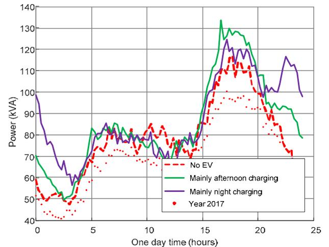
Fig. 5. Power-flow through the 160 kVA MV/LV transformer in 2030, supplying a rural network, fast EV growth and different simulation cases (3.6 kW charging power).
