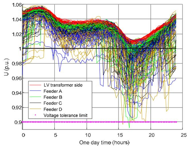
Fig. 7. Voltage profile in rural LV network in 2030, for the case of single-phase charging (3.6 kW charging power), fast EV growth and simulation case C1.
