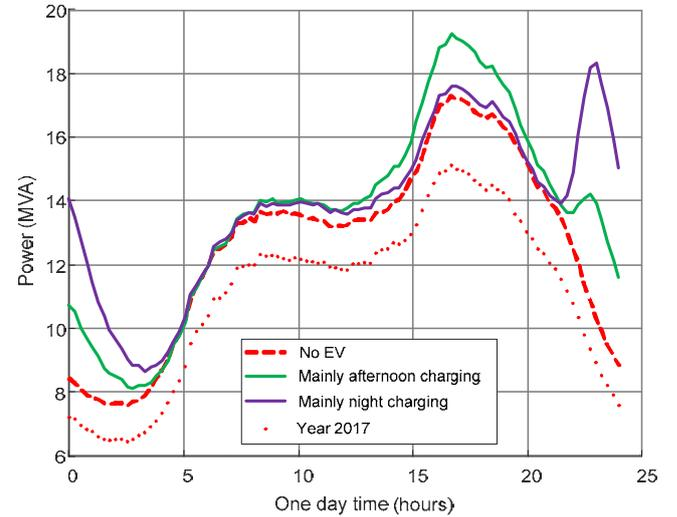
Fig. 4. Power-flow through the HV/MV transformer in 2030 for fast EV growth and different simulation cases (3.6 kW charging power).
