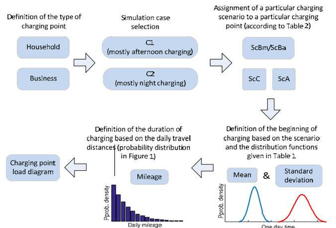
Fig. 2. Flowchart for the definition of a charging point (i.e. network node) load diagram.
