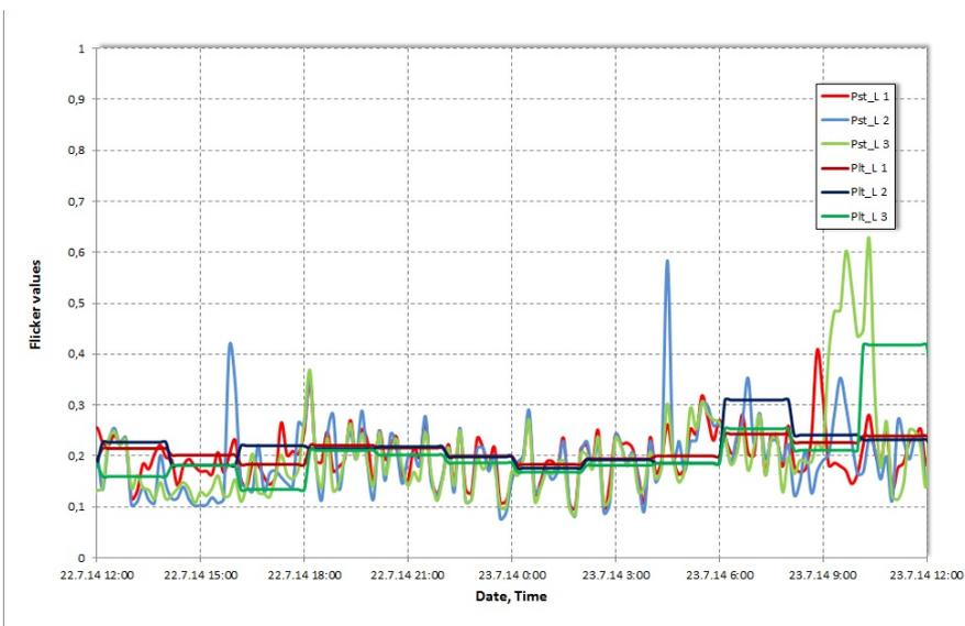
Figure 5. Measured voltage and flicker values during a 24h period 22.7.2014 to 23.7.2014. Displayed are all 3 phases.
