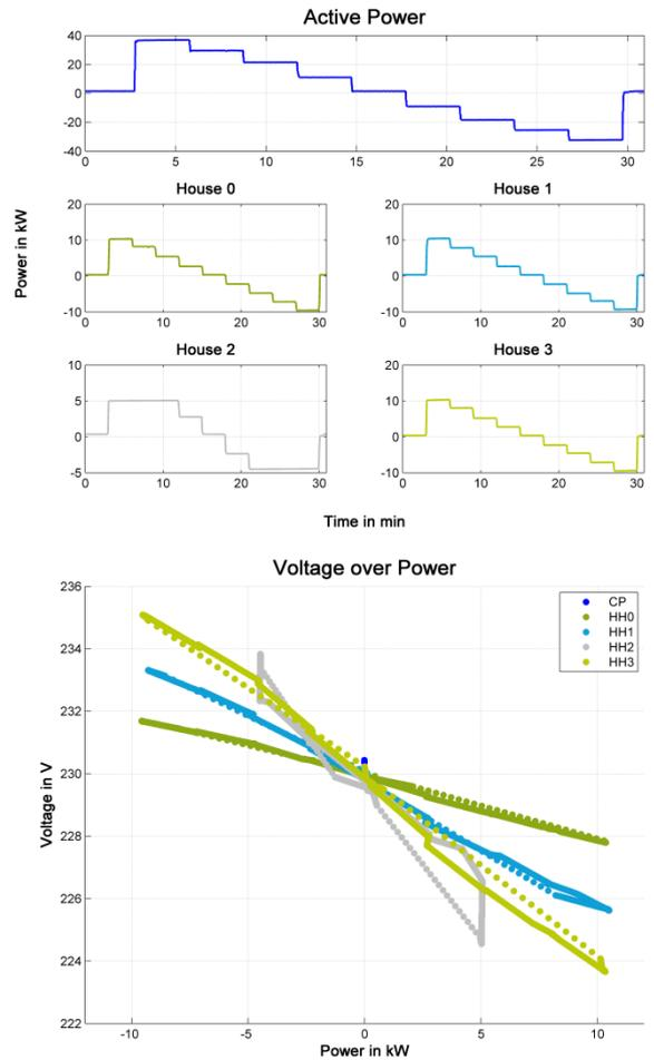
Figure 8. Voltages to power relation of a low voltage test bench
