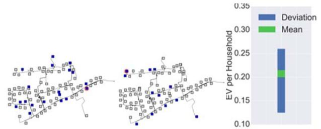
Figure 1. Determination of the electric vehicle hosting capacity of a LV network with the help of probabilistic simulations. Left: Scenario 1 voltage violation with 25 EV; Middle: Scenario 2 voltage violation with only 12 EV; Right: Estimation of hosting capacity by analysis of 50 different, randomly generated, scenarios. Each scenario is characterized by a different EV distribution.
