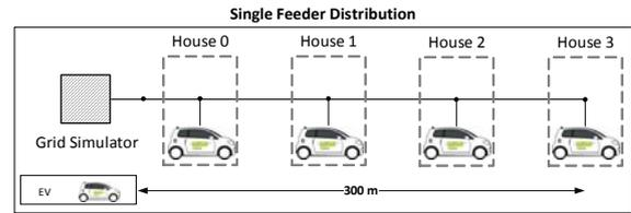
Figure 7. Setup for a single feeder with a homogeneous distribution
