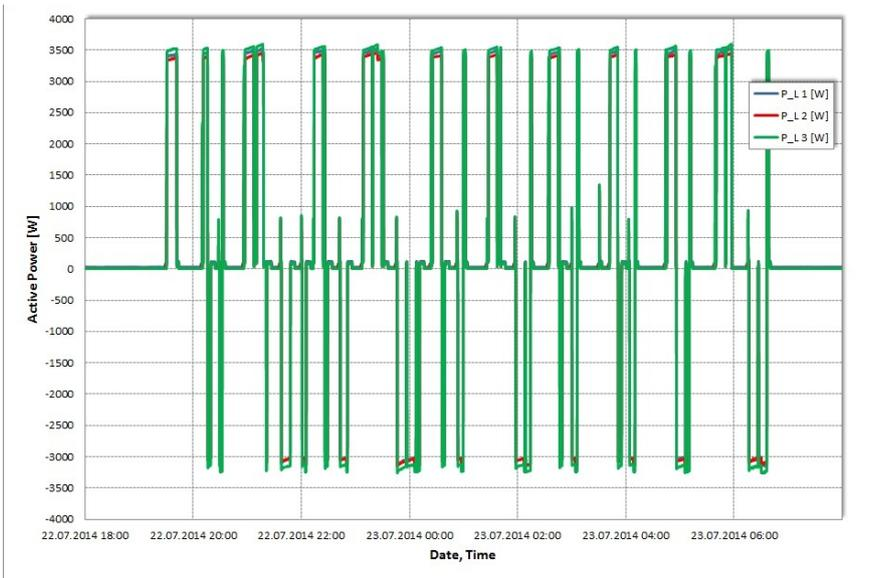
Figure 4. Provision of control reserve according to a defined charge/discharge schedule from 22.7.2014 to 23.7.2014. Displayed are all 3 phases.
