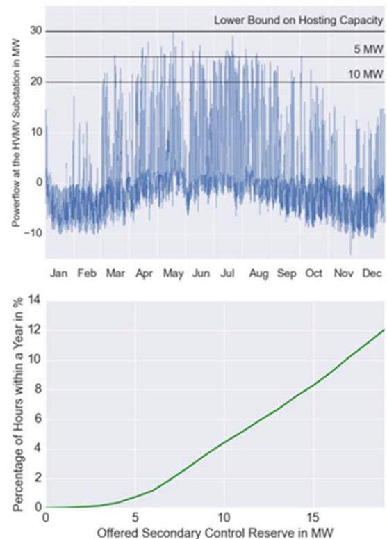
Figure 3. Top: Measured power flow over a High Voltage / Medium Voltage substation. Bottom: Percentage of hours the offered control reserve could not be provided.
