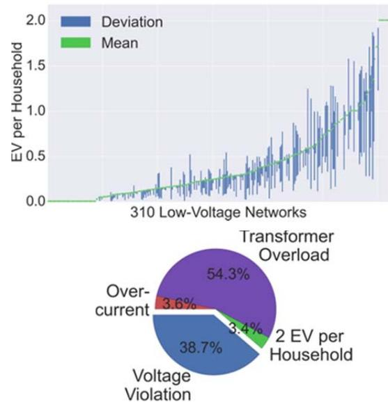
Figure 2. Hosting capacity and type of expected constraint for 310 analyzed LV networks.
