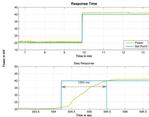
Figure 9. Experiment to analyze the dynamic settling time of the step request
