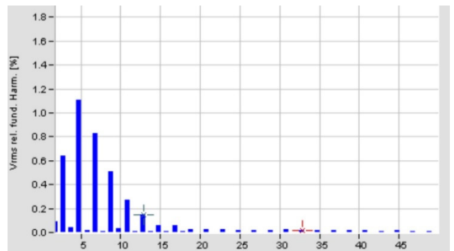
Figure 4. Background harmonic spectra of the phase voltage in % of the rms-value of the phase voltage (before starting to charge the car).
