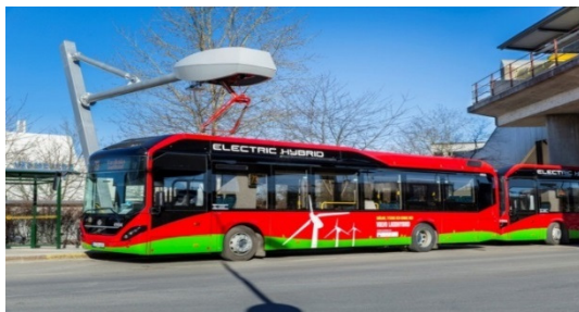
Figure 2. The hybrid bus #73 in Stockholm charged using a pantograph at the end bus stop in Ropsten.
